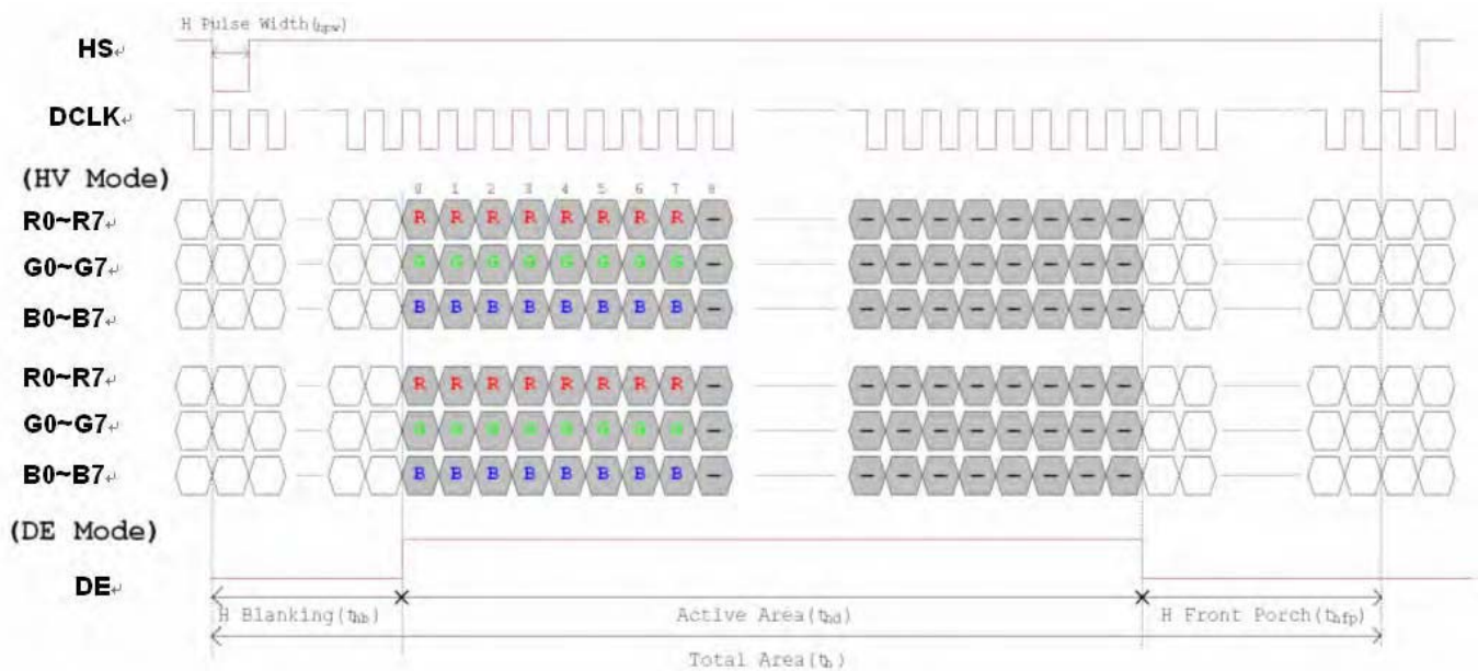
Figure 3. 1 Horizontal input timing diagram.
